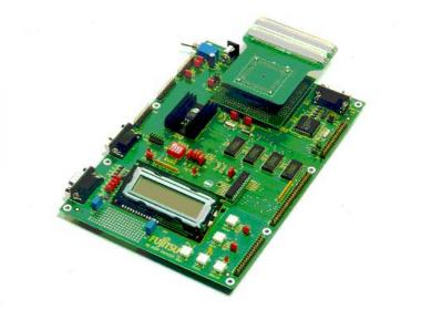
Figure 1: Using the Starterkit as target board for the ICE
